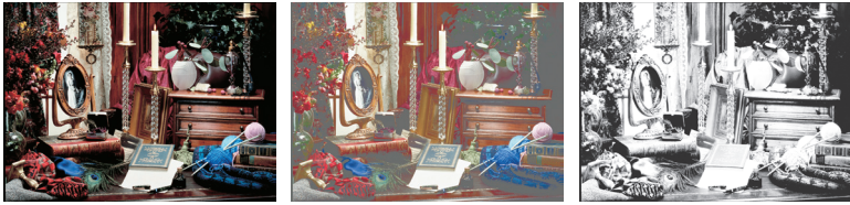
Figure 1: An image separated with undercolor removal. 4 color with 300% UCR (left), 3 color with UCR (middle), and UCR black (right).
