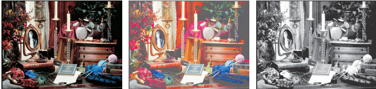
Figure 2: An image separated with gray component replacement. 4 color with 80% GCR(left), 3 color with GCR (middle), and GCR black (right).
